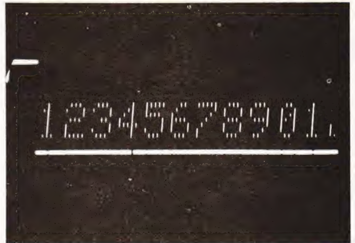
D How characters are made up on an oscilloscope display.
